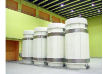
One cask providing both the storage and transport functions integrated
